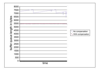
Figure 2. Buffer queue lengths with and without skew compensation
