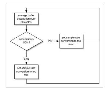
Figure 1. Skew compensation algorithm
